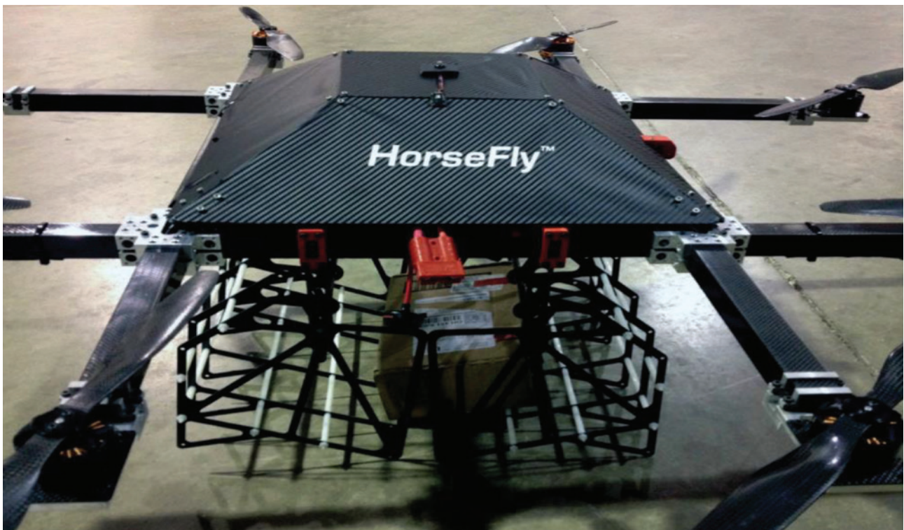
Figure 4. The Horsefly drone, developed by AMP Electric Vehicles and researchers of the University of Cincinnati, could one day help to deliver UPS packages. vi
